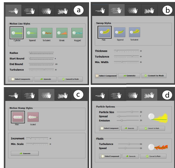
Figure 9. The four ChronoFab effect panels each include parameters for stylizing their own effects (a) Motion line (b) Sweep (c) Multiple stroboscopic stamps (d) Particle Systems .
